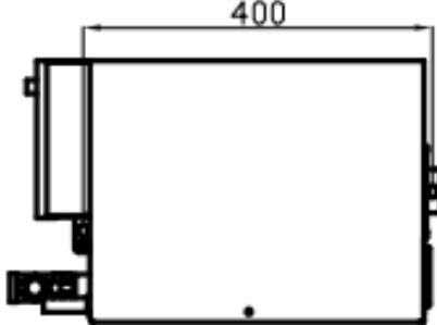
**MODEL****Cooling Capacity****Power Supply****Refrigerant****Cool/Heat Input****Sea Water Flow.****Fresh Water Flow.****Net Weight****HC24VFD****24 000 BTU****230V/50-60Hz****R32****6/8A****31L/min****21L/min****35Kg**
