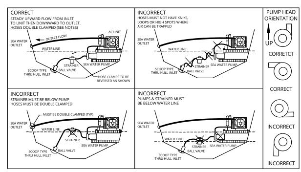
Follow the guidelines below to properly install the water system of the marine air conditioner unit.See pictures below:
