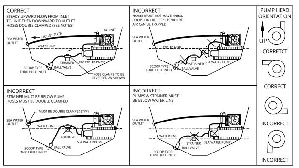
Follow the guidelines below to properly install the water system of the marine air conditioner unit. See pictures below:
