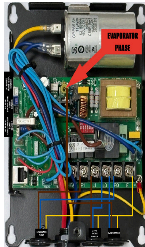
SCP electrical box with evaporator phase connection
